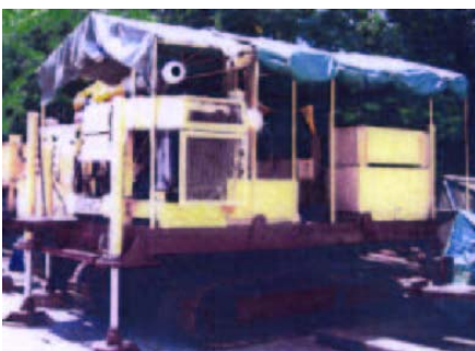
20T Kobelco Tracked CPT Rig
