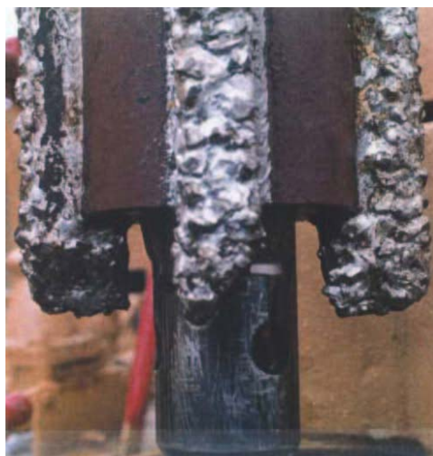
Bit shown resting on retracted wings (pushing position).
