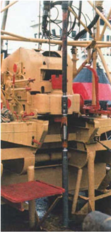
Overall view of drop push sampler unit showing (from top to bottom) stabilizer, latching unit with centralizer and sample tube.
