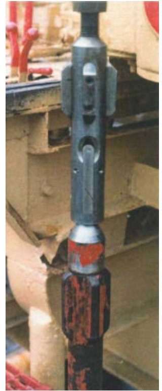
Overshot (shown latched to upper stabilizer) used to retrieve drop push sampler unit.
