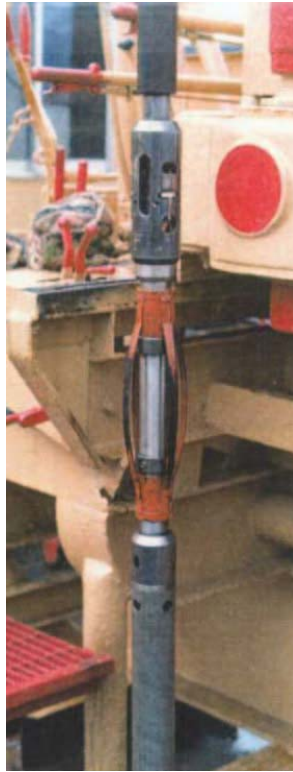
Close up of latching unit showing wings in retracted position.
