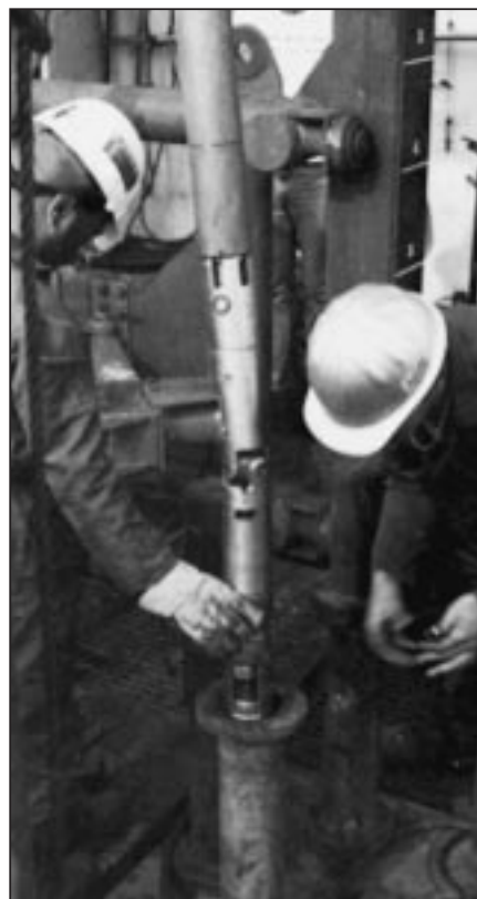
Fig. 3 - Final check of WISON in the mousehole pipe before lowering it down the drillstring
